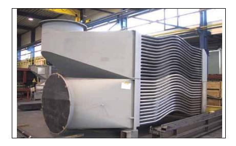
In a reheating furnace, major heat losses were found to be in the flue gases leaving the furnaces at very high temperatures. Recuperators are waste heat recovery equipments that use the energy in hot waste flue gases to preheat combustion air. The main advantages of using Recuperator for preheating the air for combustion are as under:
